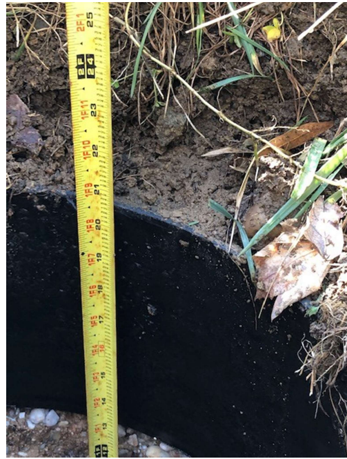
Effluent level after hydraulic loading – tank water tight – system functioning properly.
