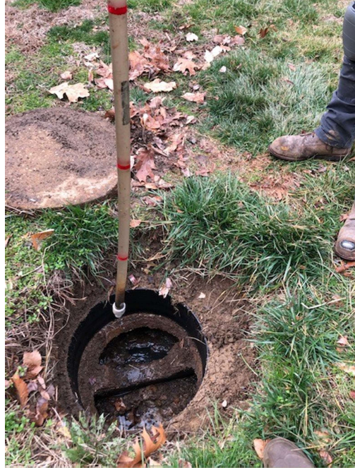
Sludge sample – 4" of sludge – 20% full.
