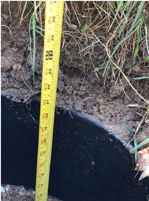
Effluent level in tank prior to hydraulic load test.
