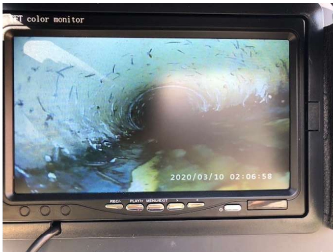
Camera used to assess drain line – no blockage – appears satisfactory.
